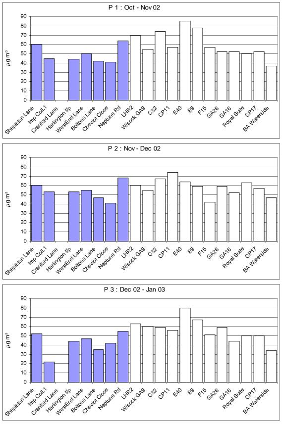
**Figures 4a-c.** Graphical representation of the bias-corrected mean  $NO_2$  concentrations. for periods 1 to 3 – in  $\mu$ g m<sup>-3</sup>.
