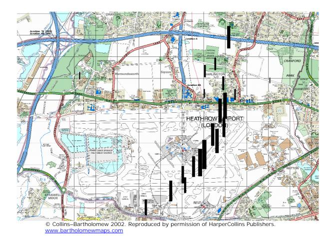
Figure 5. Geographic representation of  $NO_2$  tube bias-corrected 12-month mean results ( $\mu$ g m<sup>-3</sup>), from Oct. 02 to Oct. 03.
