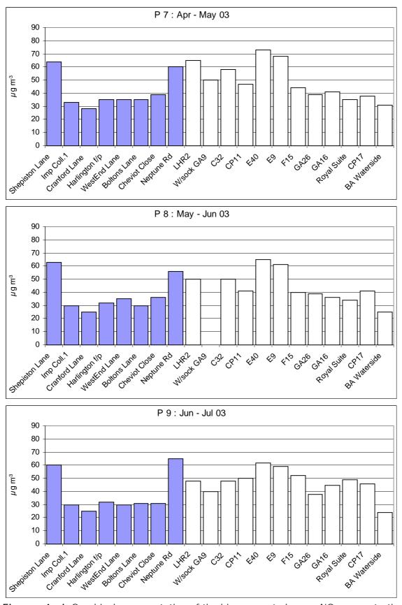
Figures 4g-i. Graphical representation of the bias-corrected mean NO<sub>2</sub> concentrations, for periods 7 to 9 – in  $\mu$ g m<sup>-3</sup>.
