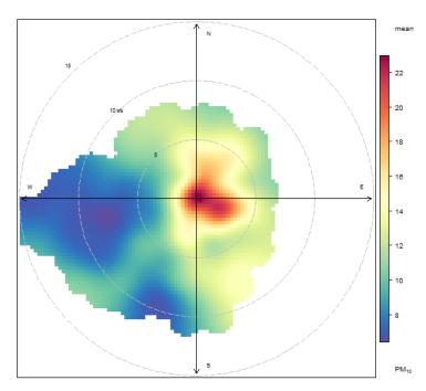
Figure 4.15 (for  $PM_{10}$ ) shows high concentrations occurred under calm conditions very close to the monitoring station (north east and south east). There was also a moderate source shown from approximately 280-290 ° for wind speeds between 5 and 10 ms<sup>-1</sup>. In contrast with the last few years, no relevant  $PM_{10}$  concentrations seem to excel for higher wind speeds.
