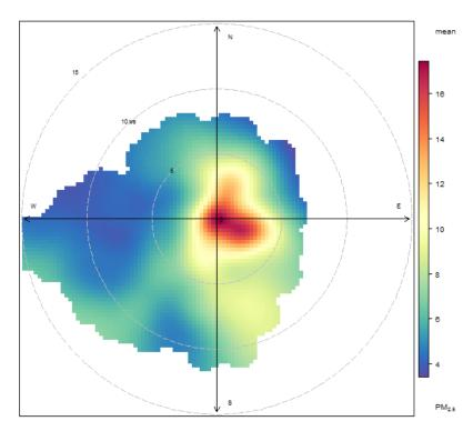
Figure 4.16 shows a similar directional pattern for  $PM_{2.5}$  to the one seen for  $PM_{10}$ . At low wind speeds, there appeared to be a build-up close to the monitoring location, suggesting the same sources were involved for both particulate size fractions. The signatures at moderate to high wind speeds were also similar, although  $PM_{2.5}$  showed a lower contribution than the ones seen for  $PM_{10}$  (note that the scales vary between Figures 4.15 and 4.16).
