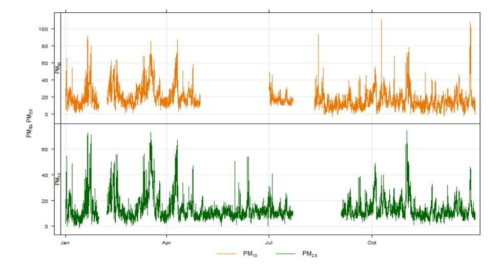
Figure 4.3 – Time series of hourly averaged concentrations of PM<sub>10</sub> and PM<sub>2.5</sub> measured by the FDMS instruments for Harlington site, 2015
