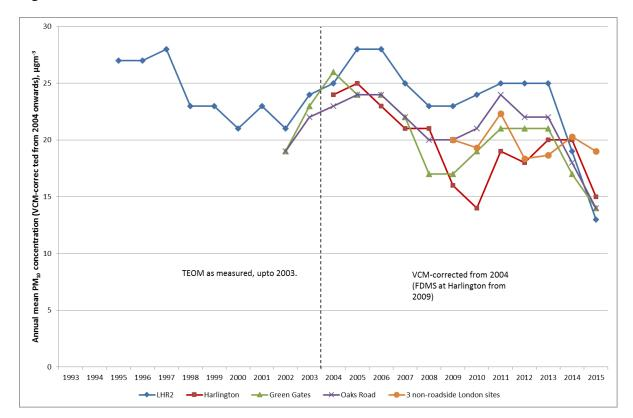
Figure 4.24 shows the annual averages of PM<sub>10</sub> collected for LHR2 since 1995 and for all sites since 2002. Data for 2015 was recorded by a FIDAS instrument, therefore requires no correction factor.
