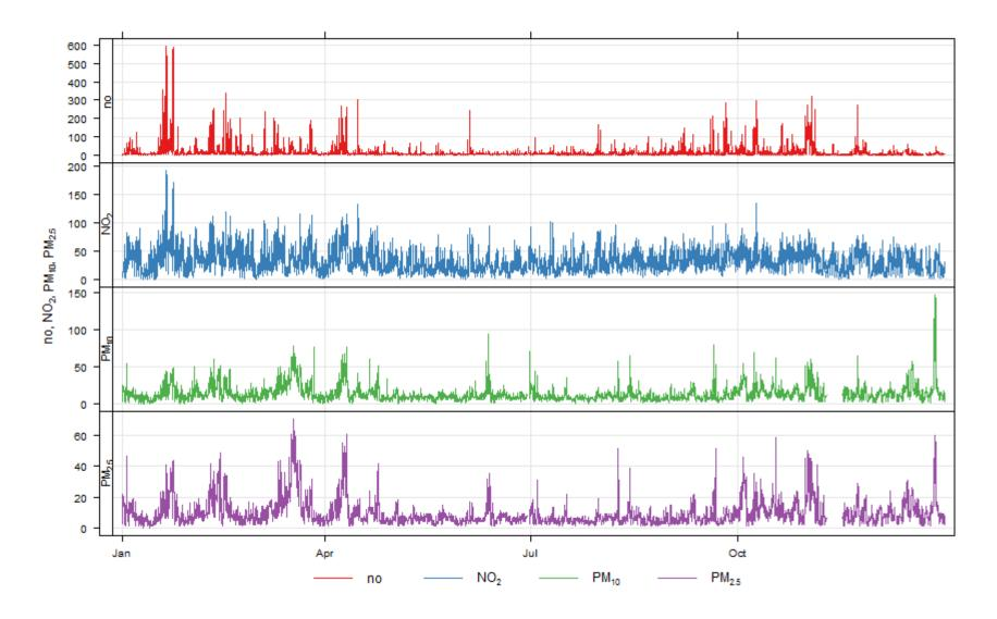
Figure 4.4 - Time series of hourly averaged concentrations of NO<sub>x</sub> and PM for Green Gates site, 2015
