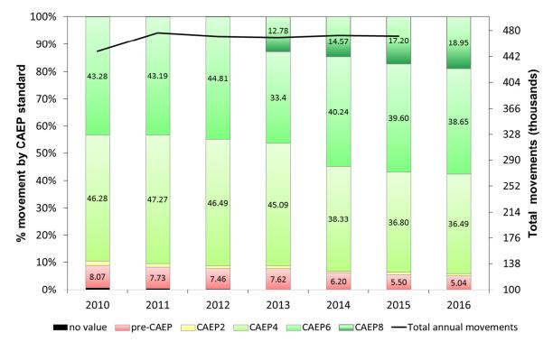
Fig.1. Total aircraft movements since 2010 by CAEP standard
